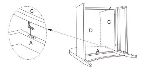
Step 3. Attach back panel (part C) to assembled unit (parts A & D) using short bolts (part G), flat washers (part J) and allen wrench (part L).
