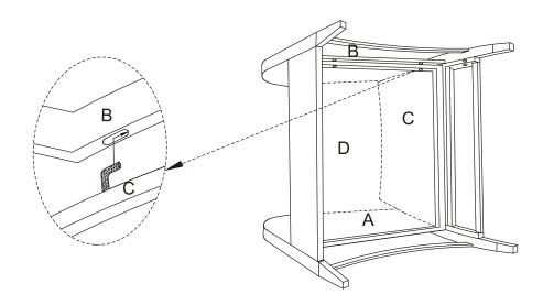
Step 5. Attach right arm panel (part B) to assembled unit (parts C & D) using short bolts (part G), long bolts (part H), flat washers (part J), hex nuts (part I), wrench (part K) and allen wrench (part L).
